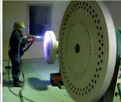
METALIZING PROCESS Use : Wind power Size : 2MW
